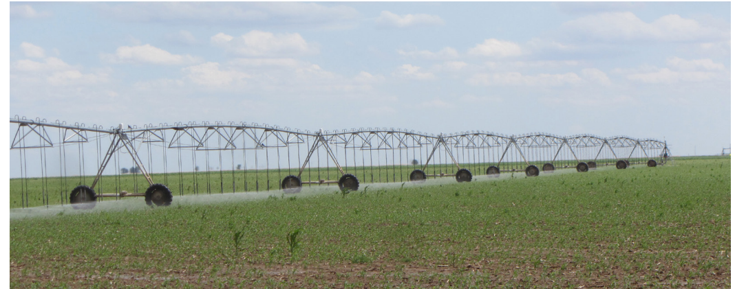
A straight pipe with water hoses spraying water rotate around a stationary spigot to irrigate crops.
